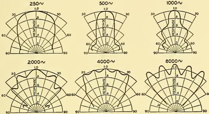
FIG. 2.13. Directional characteristics of the 15-cell cellular horn shown in Fig. 2.11A in a plane containing the line  $A-A'$  and the axis of the center horn. The polar graph depicts the pressure, at a fixed distance, as a function of the angle. The pressure for the angle  $0^\circ$  is arbitrarily chosen.
