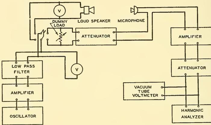
FIG. 11.11. Schematic arrangement of the apparatus for measuring the non-linear distortion of a loud speaker.
