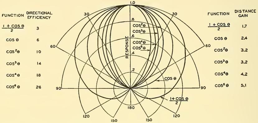
FIG. 9.41. The directional efficiency of microphones having directional characteristics which are various cosine functions. The ratio of energy response of a nondirectional microphone to the energy response of a directional microphone for sounds originating in random directions is termed directional efficiency. The ratio of the distance at which a directional microphone may be operated as compared to a nondirectional microphone is also shown.
