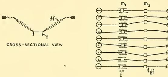
FIG. 8.12. A system consisting of a mass  $m_1$  driven by a crank at a frequency  $f$  and a second mass  $m_2$  supported by a spring coupled to  $m_1$  vibrating with a frequency  $\frac{1}{2}f$ . The cross-sectional view of the cone shows a similar system and illustrates how subharmonics may be produced by a loud speaker.
