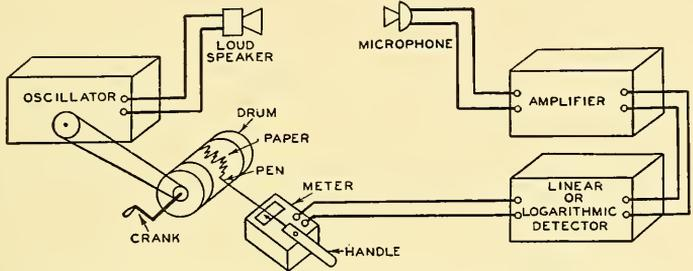
FIG. 11.6. Schematic arrangement of the apparatus for manually recording the sound pressure frequency characteristic of a sound source. (After Wolff and Ringel.)
