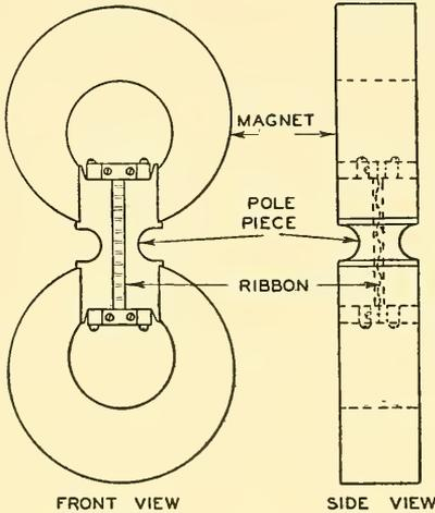
FIG. 9.13. The essential elements of a velocity microphone.
