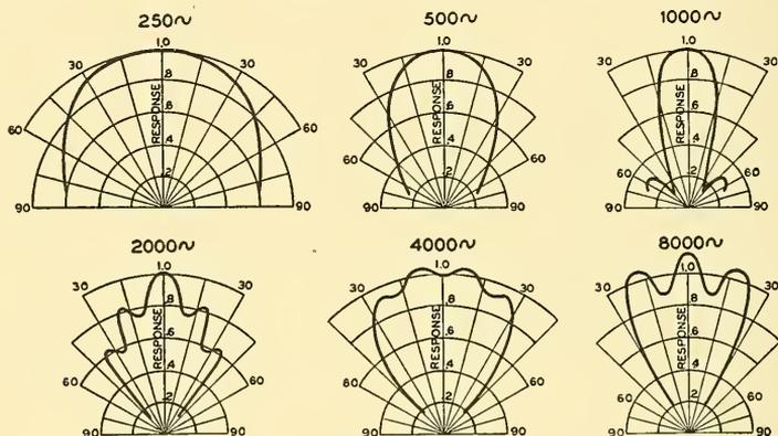
FIG. 2.12. Directional characteristics of the 15-cell cellular horn shown in Fig. 2.11*A* in a plane containing the line  $B-B'$  and the axis of the center horn. The polar graph depicts the pressure, at a fixed distance, as a function of the angle. The pressure for the angle  $0^\circ$  is arbitrarily chosen.
