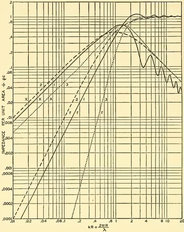
FIG. 5.1. The resistive  $r$ , and reactive  $x$ , components of the air load per unit area of the following radiators: 1. piston of radius  $R$  set in an infinite baffle; 2. a pulsating sphere of radius  $R$ ; 3. an oscillating sphere of radius  $R$ . Note: the ordinate scale of the characteristics labeled 3 must be multiplied by one-third. See Sec. 5.9.
