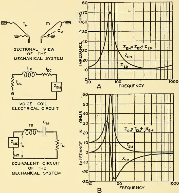
FIG. 7.3. Electrical and mechanical circuits of a dynamic loud speaker at the low frequencies. The normal impedance,  $Z_{EN}$ , and the blocked impedance,  $Z_{ED}$ , characteristics of the voice coil of a typical dynamic loud speaker are shown in graph A. The characteristics of the resistive,  $r_{EM}$ , and the reactive  $x_{EM}$ , components of the motional impedance  $Z_{EM}$  are shown in graph B.
