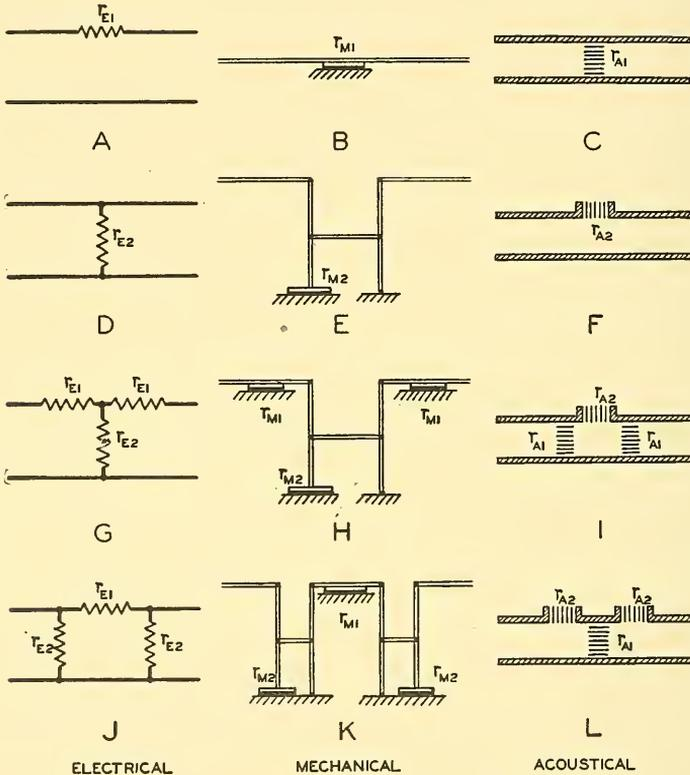
FIG. 4.7. A— an electrical resistance in series with a line. The mechanical and acoustical equivalents are shown in B and C. D an electrical resistance in shunt with a line. The mechanical and electrical equivalents are shown in E and F. A “T” and “ $\pi$ ” electrical resistance network are shown in G and J. The mechanical and acoustical equivalents are shown in H, I, K and L.
