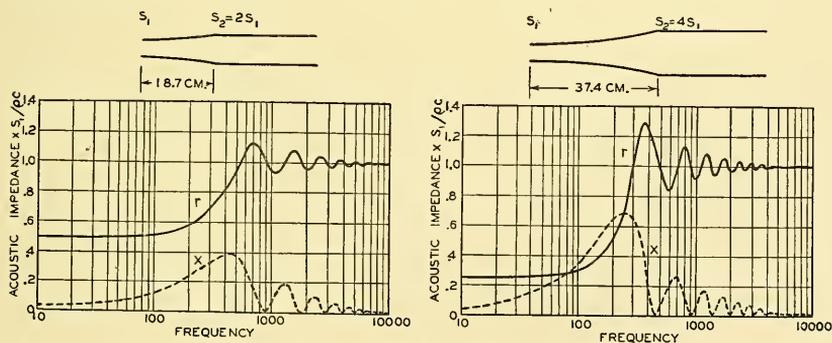
FIG. 5.7. The throat acoustic impedance characteristics of two exponential connectors with a flare cutoff of 100 cycles. The mouth of the horn is connected to an infinite pipe.  $r$ , resistive component.  $x$ , reactive component.
