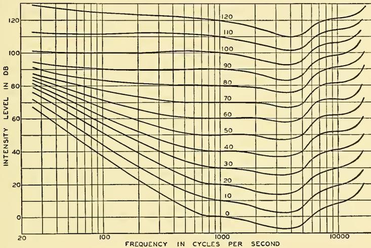
FIG. 13.1. Contour lines of equal loudness for normal ears. Numbers on curves indicate loudness level. 0 db =  $10^{-16}$  watts per square centimeter. 0 db = 0.000204 dyne per square centimeter. (After Fletcher and Munson.)
