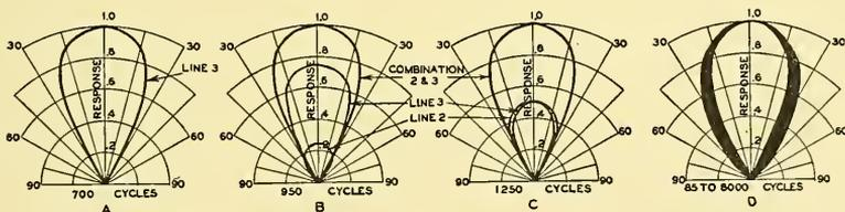
FIG. 9.40. A. The directional characteristic of line 3 at 700 cycles. B. The directional characteristics of lines 2 and 3 and the resultant at 950 cycles. C. The directional characteristics of lines 2 and 3 and the resultant of 1250 cycles. D. The directional characteristics of the microphone shown in Fig. 9.38 for the range from 85 to 8000 cycles fall within the shaded area.
