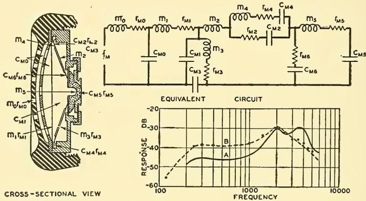
FIG. 9.2. Cross-sectional view and equivalent circuit of an improved single button carbon microphone. The open circuit voltage response characteristics are shown by the graph. *A*. Response in free space. *B*. Response for constant sound pressure on the diaphragm. Dots computed from equivalent circuit. (After Jones.)
