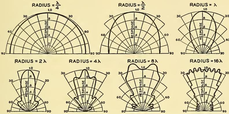
FIG. 2.4. Directional characteristics of a  $60^\circ$  arc as a function of the radius and the wavelength. The polar graph depicts the pressure, at a large fixed distance, as a function of the angle in the plane of the arc. The pressure for the angle  $0^\circ$  is arbitrarily chosen as unity.
