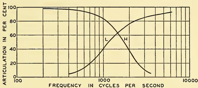
FIG. 13.8. The effect of the frequency range upon the articulation of speech. *H.* High pass filter — all frequencies below the frequency given by the abscissa removed. *L.* Low pass filter — all frequencies above the frequency given by the abscissa removed. (After Fletcher "Speech and Hearing," D. Van Nostrand Co.)
