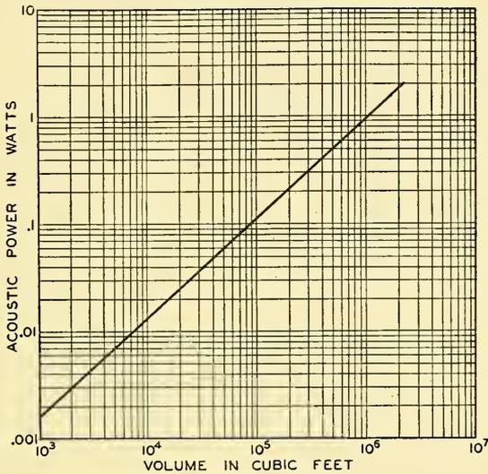
FIG. 12.7. Acoustic power required to produce an intensity level of 80 db as a function of the volume of the auditorium.
