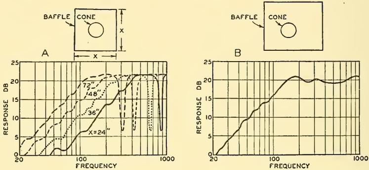
FIG. 7.8. *A.* Pressure response frequency characteristics of a mass controlled direct radiator dynamic loud speaker mounted in 2-, 3-, 4- and 6-foot square baffles. *B.* Response frequency characteristic of a mass controlled direct radiator dynamic loud speaker mounted in an irregular baffle.
