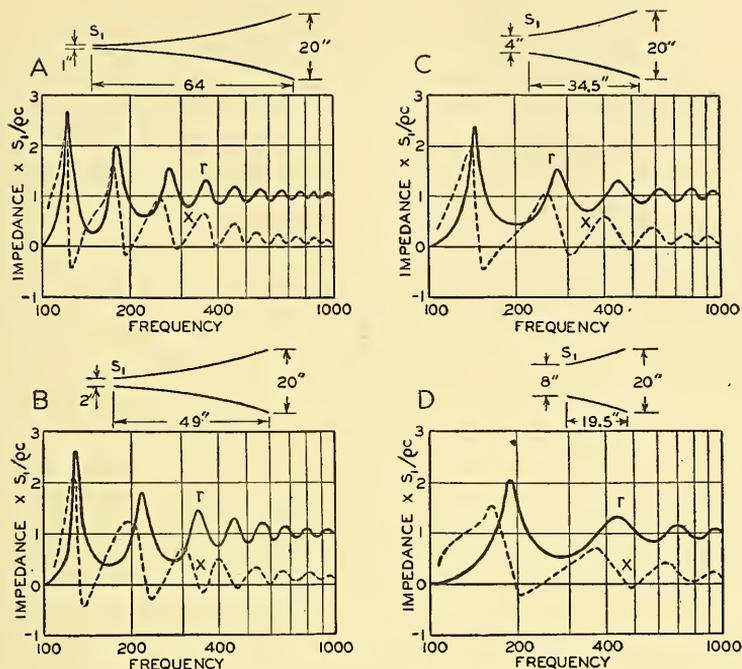
FIG. 5.6. The throat impedance characteristics of a group of exponential horns, with a flare cutoff of 100 cycles and a mouth diameter of 20 inches, as a function of the throat diameter.  $S_1$  is the area of the throat in square centimeters. Note: the characteristic shown is the throat acoustic impedance multiplied by  $S_1$  and divided by  $\rho c$ .  $r$ , resistive component.  $x$ , reactive component.
