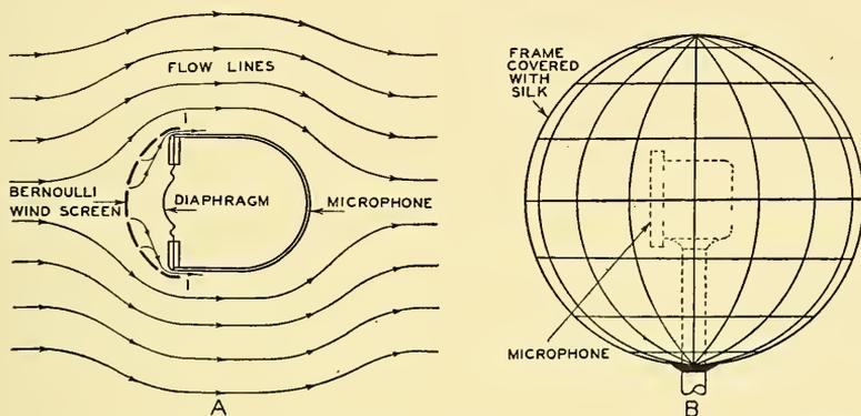
FIG. 9.42. Wind screens for microphones. *A*. Bernoulli wind screen applied to a dynamic microphone. *B*. Wind screen consisting of a wire frame covered with sheer silk.
