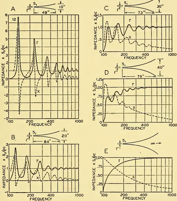
FIG. 5.5. The throat impedance characteristics of a group of exponential horns, with a flare cutoff of 100 cycles and a throat diameter of 1 inch, as a function of the mouth diameter.  $S_1$  is the area of the throat in square centimeters. Note: the characteristic shown is the throat acoustic impedance multiplied by  $S_1$  and divided by  $\rho c$ .  $r$ , resistive component.  $x$ , reactive component.
