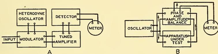
FIG. 11.12. Harmonic analyzers. *A.* Heterodyne analyzer. *B.* Balance bridge analyzer.
