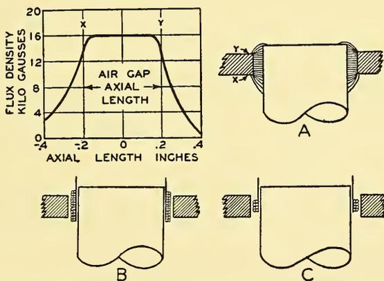
FIG. 8.11. Graph of the flux distribution in an air gap. *A.* Typical distribution of the flux lines in an air gap. *B.* A voice coil longer than the air gap. *C.* A voice coil shorter than the air gap.
