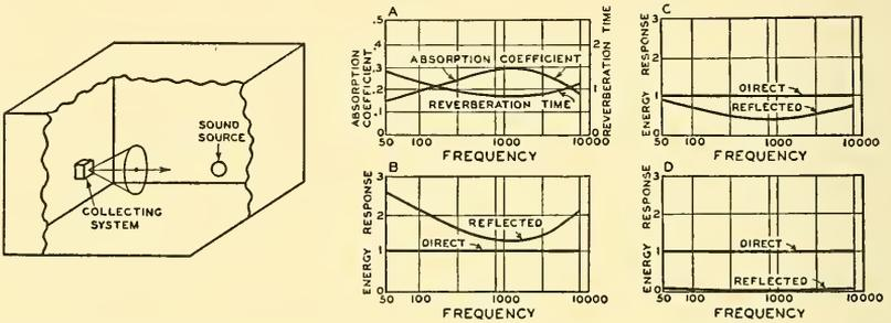
FIG. 12.14. Sound collecting system in a studio. Graph *A* shows the reverberation time and the absorption coefficient of the boundaries of a typical studio. Graphs *B*, *C* and *D* show the energy response for the direct and reflected sounds for various microphones as follows: *B*. Nondirectional microphone. *C*. Bidirectional velocity or unidirectional microphone. *D*. Ultradirectional microphone.
