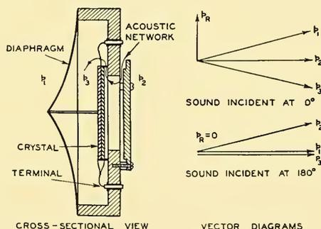
FIG. 9.30. Crystal unidirectional microphone employing a phase shifting network. The vector diagram depicts the magnitude and phase available for driving the diaphragm for  $0^\circ$  and  $180^\circ$ .
