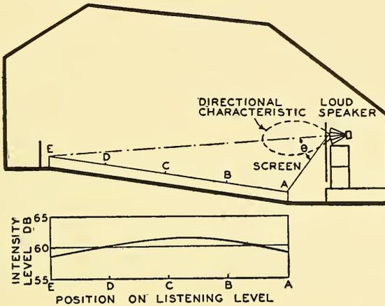
FIG. 12.2. Arrangement of the loud speaker for a sound motion picture reproducing system in a theatre. The graph shows the intensity level at points along the listening level.
