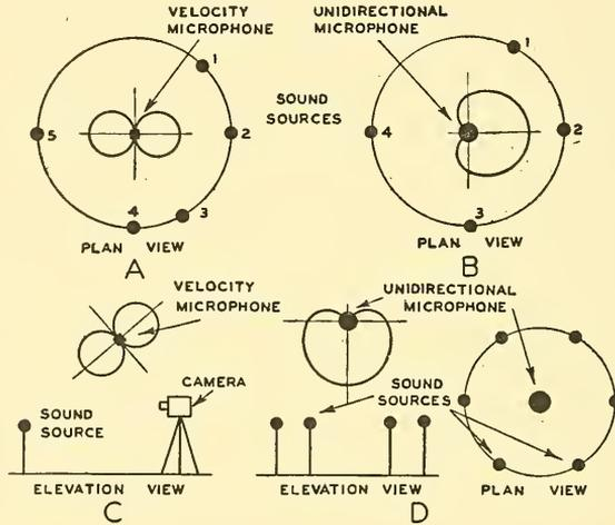
FIG. 12.15. Examples illustrating the use of directional microphones.
