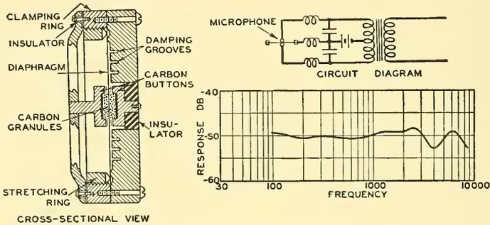
FIG. 9.3. Cross-sectional view and electrical circuit diagram of a double button, stretched diaphragm, carbon microphone. The graph shows the open circuit voltage response frequency characteristic for constant sound pressure on the diaphragm.
