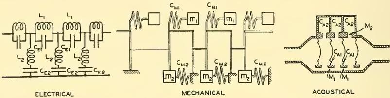
FIG. 4.12. Band elimination wave filters.
