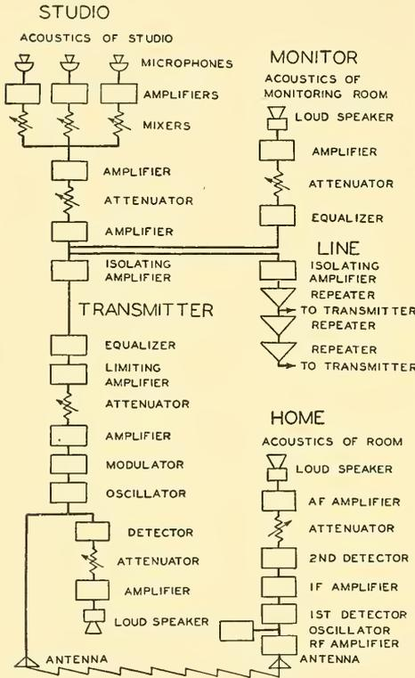
FIG. 12.21. Complete radio broadcasting and receiving system.
