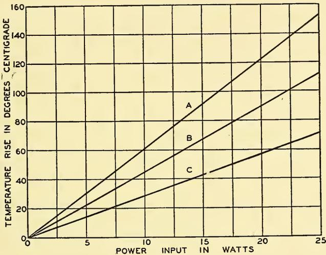
FIG. 8.13. The temperature rise as a function of the power delivered to a voice coil for air gap clearances as follows: A. 0.021 inch, B. 0.015 inch, C. 0.009 inch. Coil  $1\frac{1}{2}$  inch in diameter and 0.25 inch in length.
