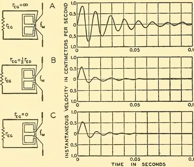
FIG. 7.16. The transient response of a 12-inch loud speaker to a unit force for various types of generators. *A.* Generator of very high resistance. *B.* Generator having a resistance of one-half of the loud speaker impedance. *C.* Generator of zero impedance.
