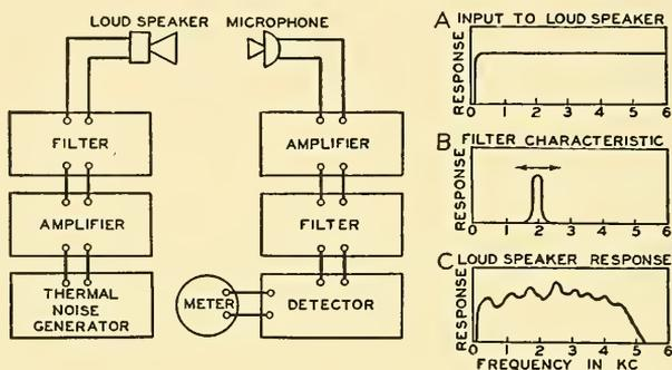
FIG. 11.9. Schematic arrangement of the apparatus employing a thermal noise generator and a band pass filter for obtaining the response frequency characteristic of a loud speaker *A*. Input to the loud speaker. *B*. The response frequency characteristic of the band pass filter. *C*. Response frequency characteristic of the loud speaker.
