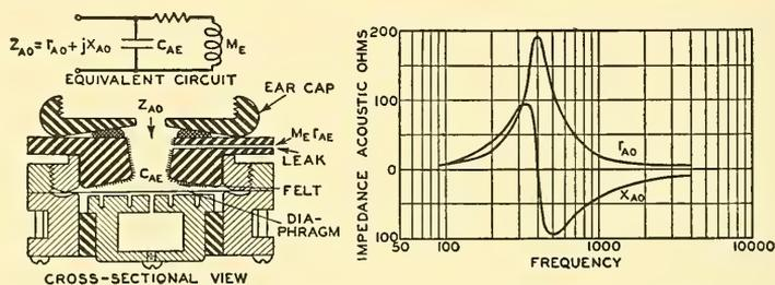
FIG. 11.15. A cross-sectional view of an artificial ear employing a standard condenser microphone and the equivalent electrical circuit of the acoustical system. The graph shows the resistive  $r_{AO}$  and reactive  $X_{AO}$  components of the acoustic impedance, looking into the aperture of the ear cap, as a function of the frequency.  $C_{AE}$  acoustic capacitance of the cavity.  $M_E$  and  $r_{AE}$  inductance and acoustic resistance of the leak.
