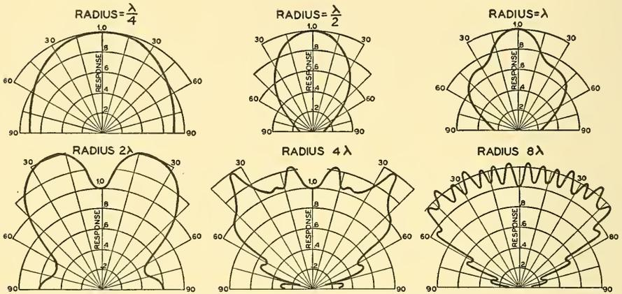
FIG. 2.6. Directional characteristics of a  $120^\circ$  arc as a function of the radius and the wavelength. The polar graph depicts the pressure, at a large fixed distance, as a function of the angle in the plane of the arc. The pressure for the angle  $0^\circ$  is arbitrarily chosen as unity.
