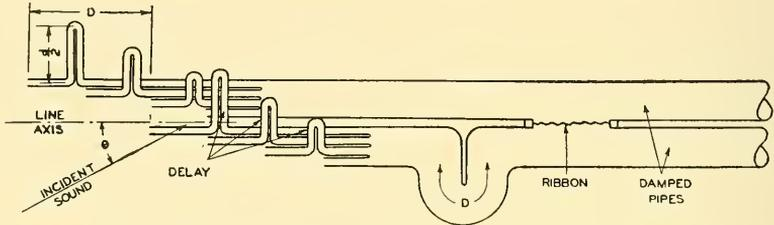
FIG. 9.36. Line Microphone. Useful directivity on the line axis. This microphone consists of two lines of the type shown in Fig. 9.34 displaced by a distance  $D$  along the axis. In the line nearest the ribbon element a bend is inserted which introduces a path length  $D$ . The ribbon element measures the difference in pressure in the two lines.
