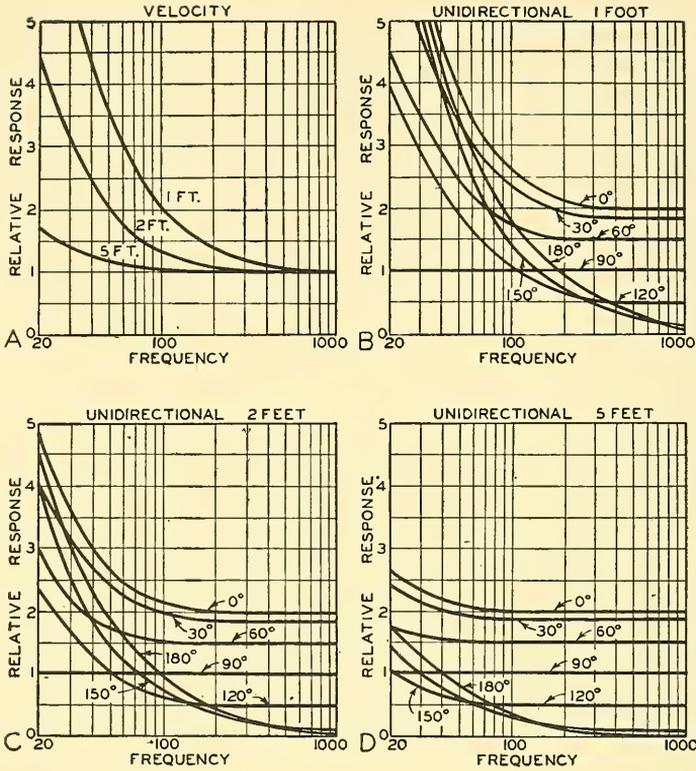
FIG. 9.26. *A*. The relative voltage output of a velocity (or pressure gradient) microphone as compared to a nondirectional pressure microphone for distances of 1, 2 and 5 feet. *B*, *C*, *D*, the relative voltage output of a unidirectional microphone as compared to a nondirectional pressure microphone for distances of 1, 2 and 5 feet and for various angles of the incident sound.
