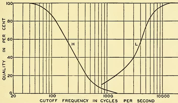
FIG. 13.9. The effect of the frequency range upon the quality of orchestra music. *H.* High pass filter — all frequencies below the frequency given by the abscissa removed. *L.* Low pass filter — all frequencies above the frequency given by the abscissa removed. (After Snow.)
