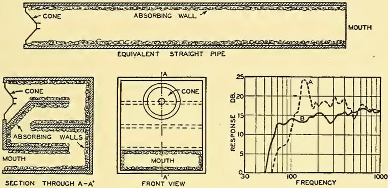
FIG. 7.12. Acoustical labyrinth loud speaker. The equivalent straight axis damped pipe is shown above. The pressure response characteristic of the labyrinth loud speaker is labeled *B* on the graph. The pressure response characteristic of the corresponding cabinet loud speaker is labeled *A* on the graph. (After Olney.) (Courtesy of The Blakiston Company from Olson and Massa, "Applied Acoustics.")
