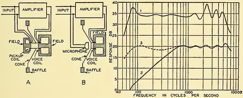
FIG. 7.14. Loud speaker and amplifier feedback systems. *A*. The output of the pickup coil is fed into the input side of the amplifier. *B*. The output of the microphone is fed into the input side of the amplifier. The graph shows the pressure response characteristics of system *A*: 1. without feedback, 2. with feedback, 3. with feedback and compensation.
