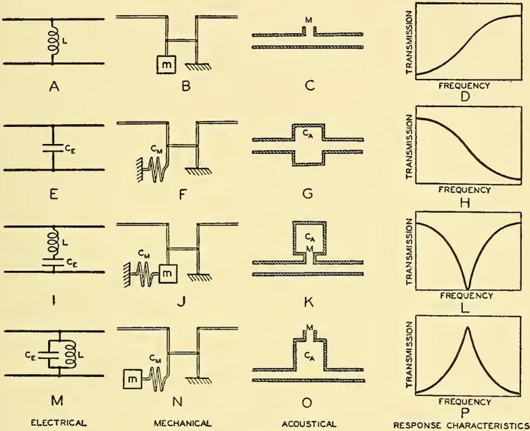
FIG. 4.5. A line shunted by the following: *A* an inductance. *E* a capacitance. *I* an inductance and a capacitance in series. *M* an inductance and a capacitance in parallel. The mechanical equivalents are shown in *B*, *F*, *J* and *N*. The acoustical equivalents are shown in *C*, *G*, *K* and *O*. The transmission-frequency characteristics are shown in *D*, *H*, *L* and *P*.
