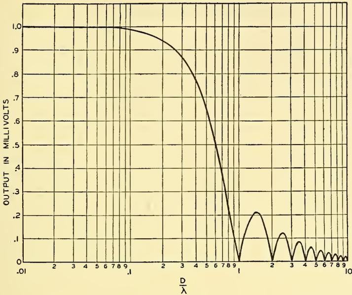
FIG. 9.11. Computed open circuit voltage response frequency characteristic of a pressure gradient, mass controlled, electrodynamic microphone.
