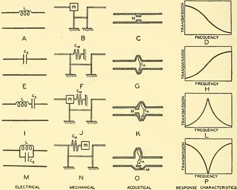
FIG. 4.6. A line in series with the following: *A* an inductance. *E* a capacitance. *I* an inductance and a capacitance in series. *M* an inductance and a capacitance in parallel. The mechanical equivalents are shown in *B*, *F*, *J* and *N*. The acoustical equivalents are shown in *C*, *G*, *K* and *O*. The transmission-frequency characteristics are shown in *D*, *H*, *L* and *P*.
