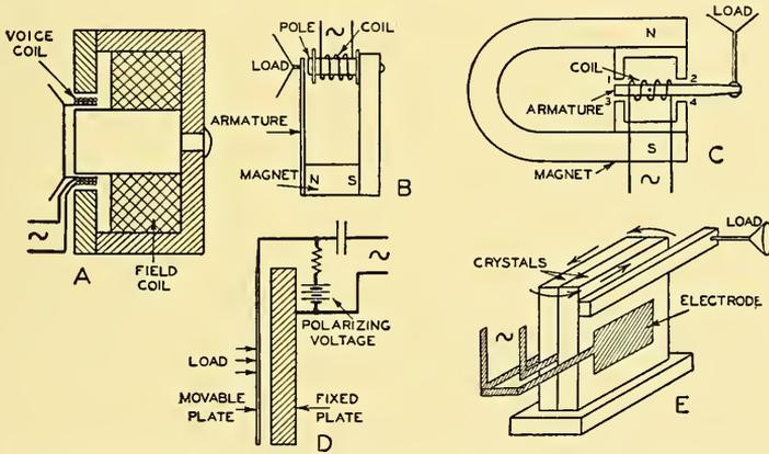
FIG. 6.1. Driving systems: *A* electrodynamic, *B* electromagnetic, reed armature, *C* electromagnetic, balanced armature, *D* condenser, *E* crystal.
