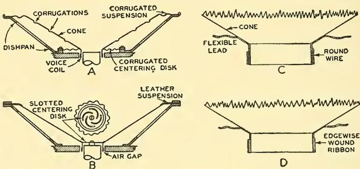
FIG. 7.18. Cones and voice coils. Sectional views. *A*. Felted paper cone. *B*. Developed paper cone with leather outside suspension. *C*. Voice coil wound with round wire. *D*. Voice coil with edgewise wound ribbon.
