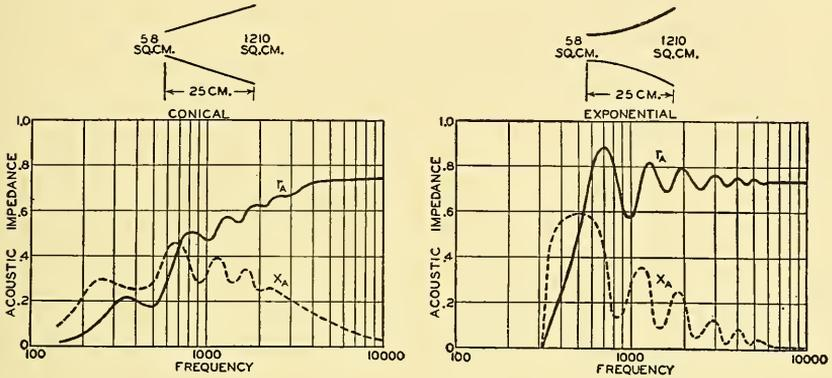
FIG. 5.4. Throat acoustic impedance characteristics of a conical and an exponential horn having the same throat and mouth area.  $r_A$ , resistive component.  $x_A$ , reactive component.
