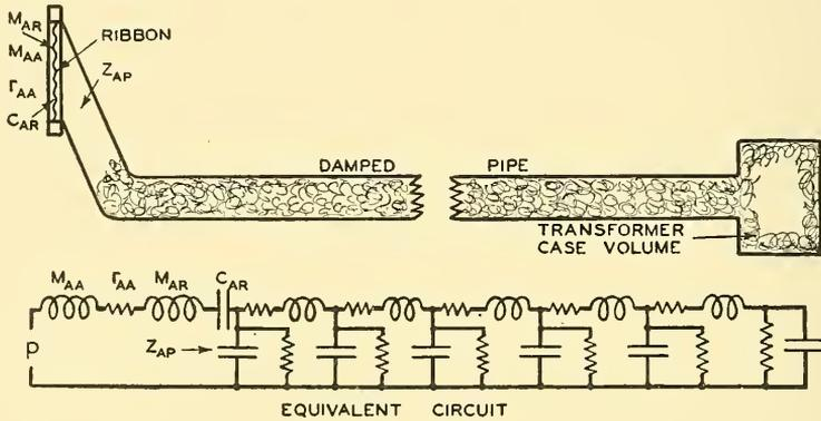
FIG. 9.8. The elements of the pressure microphone and the equivalent electrical circuit of the acoustical system.  $M_{AR}$  inductance of the ribbon.  $C_{AR}$  acoustic capacitance of the ribbon.  $r_{AA}$  acoustic resistance of the air load on the ribbon.  $M_{AA}$  inductance of the air load upon the ribbon.  $Z_{AP}$  acoustic impedance of the pipe terminating the ribbon.  $p$  driving sound pressure.
