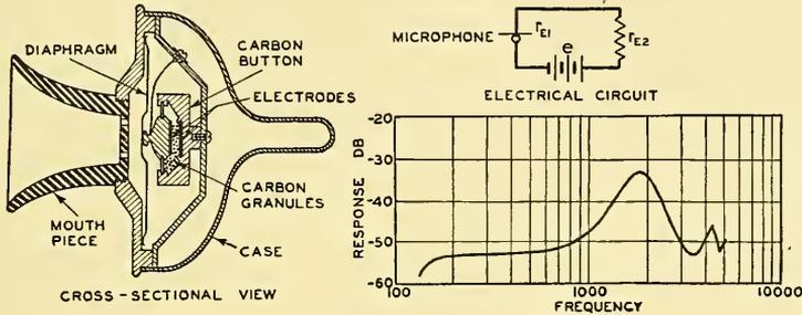
FIG. 9.1. Cross-sectional view and the electrical circuit diagram of a single button carbon microphone. The graph shows the free space open circuit voltage response frequency characteristic.
