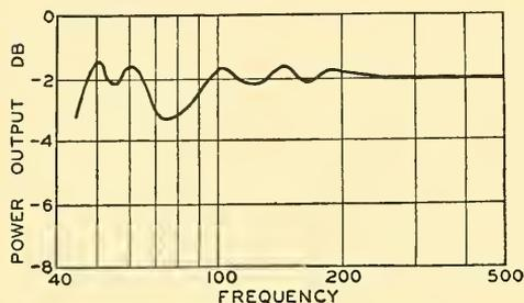
FIG. 8.5. Power output characteristic of the horn (Fig. 5.6B with all dimensions multiplied by  $2\frac{1}{2}$ ) coupled to a  $10\frac{1}{2}$ -inch diameter, 10-gram diaphragm driven by a 5-gram aluminum voice coil in a field of 20,000 gauss. Damped resistance of voice coil, 20 ohms. Impedance of vacuum tube through a transformer, 35 ohms.
