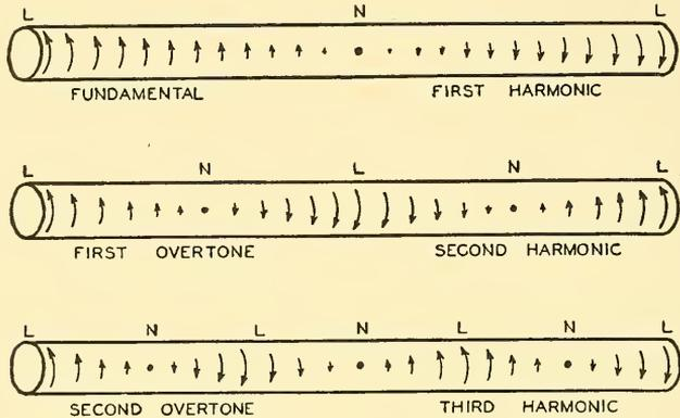
FIG. 3.6. Modes of torsional vibration of a free rod. The nodes and loops are indicated by *N* and *L*.
