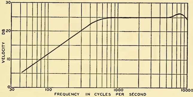
FIG. 10.7. Velocity response frequency characteristic of a phonograph record with constant voltage applied to an equalized recording amplifier.
