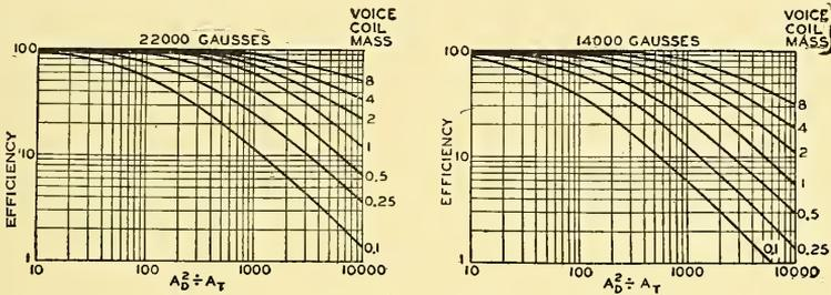
FIG. 8.2. The initial efficiency of a horn loud speaker as a function of  $A_D^2/A_T$  for aluminum voice coils having masses of 0.1, 0.25, 0.5, 1.2, 4, and 8 grams and flux densities of 22,000 and 14,000 gauss.  $A_D$  and  $A_T$  are the areas of the diaphragm and throat, respectively, in square centimeters. The above graphs may be applied to a copper voice coil by multiplying the ratio  $A_D^2 \div A_T$  by one-half.
