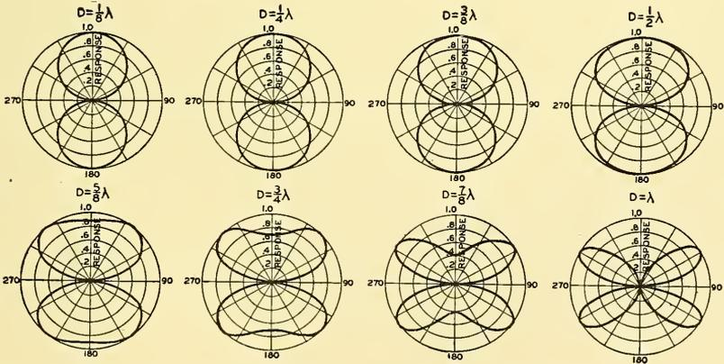
FIG. 9.12. Directional characteristics of a pressure gradient microphone as a function of the dimensions and the wavelength. The polar graph depicts the output, in volts, as a function of the angle, in degrees. The maximum response is arbitrarily chosen as unity.
