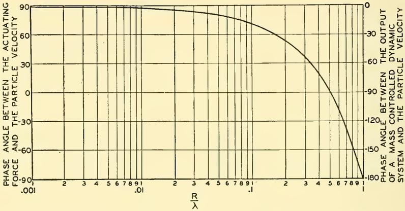
FIG. 9.22. The phase angle, in degrees, between the actuating force and the particle velocity for a mass controlled ribbon with a circular baffle as a function of  $R/\lambda$ . The phase angle between the voltage output of a mass controlled electrodynamic ribbon located in a magnetic field as a function of  $R/\lambda$ .
