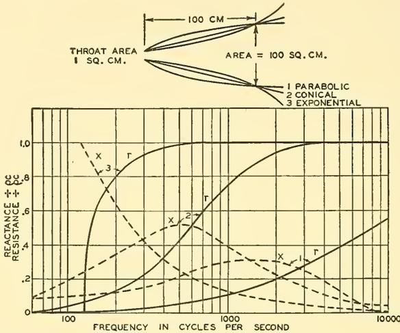
FIG. 5.3. Throat resistance  $r$ , and reactance  $x$ , of infinite parabolic, conical and exponential horns having the same throat area and the same cross section at a distance of 100 centimeters from the throat.
