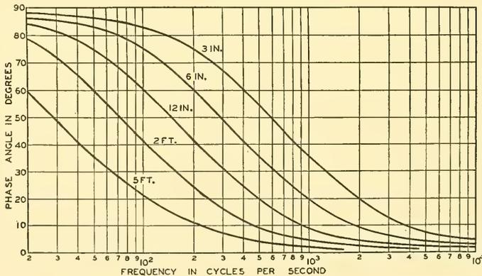
FIG. 1.2. Phase angle between the pressure and particle velocity in a spherical sound wave for distances of  $\frac{1}{3}$ ,  $\frac{1}{2}$ , 1, 2 and 5 feet from the source. (Courtesy of The Blakiston Company from Olson and Massa, Applied Acoustics.)
