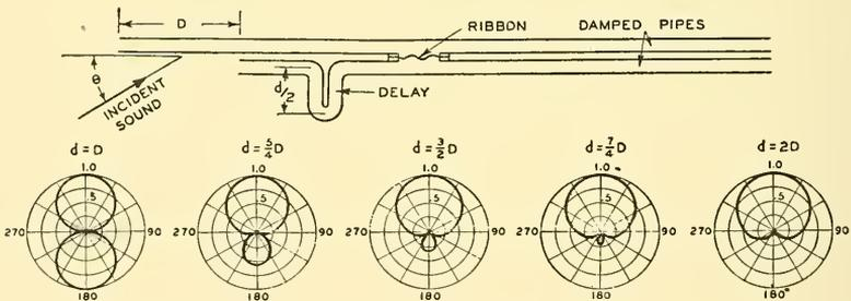
FIG. 9.29. A directional microphone employing a phase shifting system. The polar graphs show the directional characteristics for various ratios of  $d/D$ . The polar graph depicts the output, in volts, as a function of the angle, in degrees. The maximum response is arbitrarily chosen as unity.
