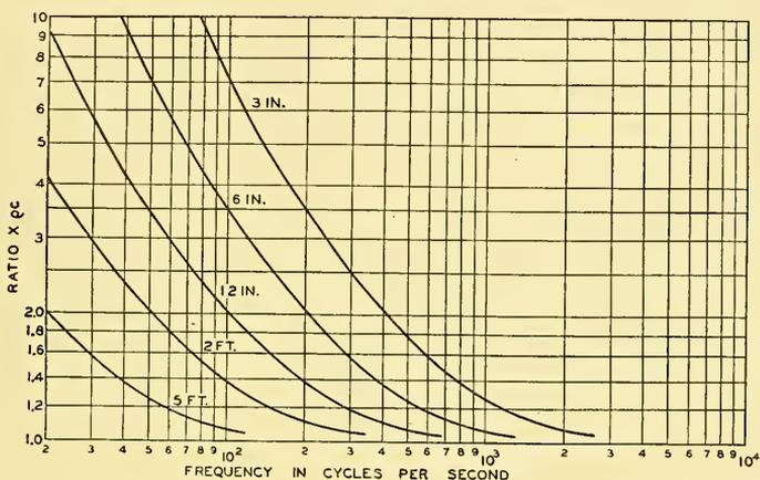
FIG. 1.3. Ratio of the absolute magnitude of the particle velocity to the pressure in a spherical sound wave for distances of  $\frac{1}{4}$ ,  $\frac{1}{2}$ , 1, 2 and 5 feet from the source. (Courtesy of The Blakiston Company from Olson and Massa, Applied Acoustics.)
