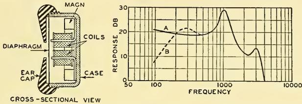
FIG. 10.1. Cross-sectional view of a bipolar telephone receiver. The graph shows the pressure response frequency characteristics. *A*. Receiver feeding a closed cavity. *B*. Receiver feeding an artificial ear.
