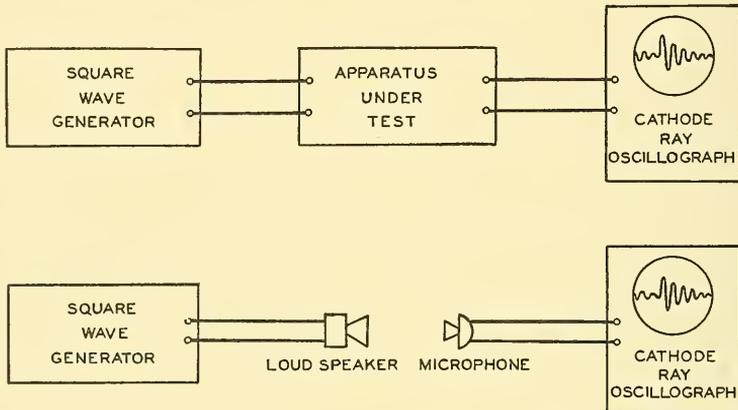
FIG. 11.14. Schematic arrangement of the apparatus employing a square wave generator and a cathode ray tube for indicating the transient response characteristics of acoustical apparatus such as microphones or loud speakers.
