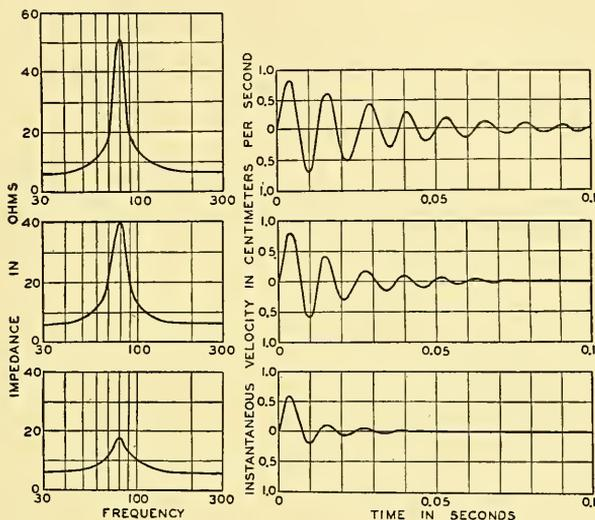
FIG. 7.17. The unit force response of a loud speaker coupled to a generator of very high resistance for different values of the internal mechanical resistance. The impedance frequency characteristics indicate the degree of internal damping.
