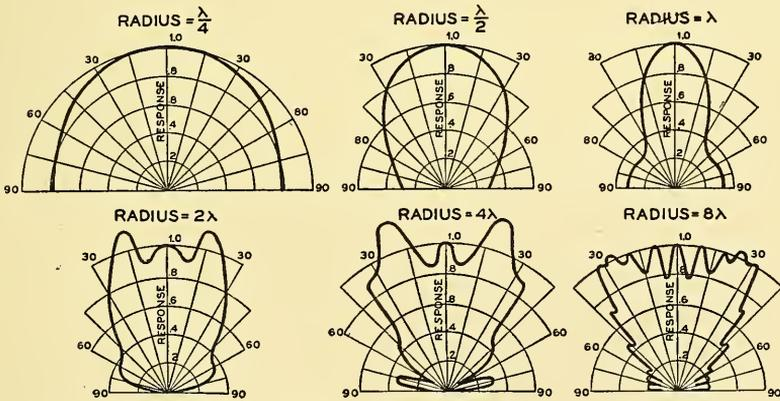
FIG. 2.5. Directional characteristics of a  $90^\circ$  arc as a function of the radius and the wavelength. The polar graph depicts the pressure at a large fixed distance, as a function of the angle in the plane of the arc. The pressure for the angle  $0^\circ$  is arbitrarily chosen as unity.
